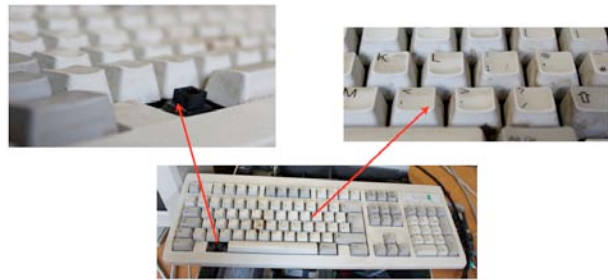
Figure 27: Dirtiness and physical deterioration in the computer's keyboard.
