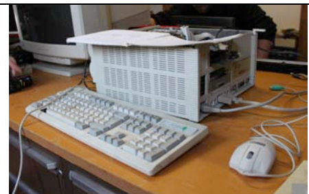
Figure 14: The monitor and camera cables must be connected to the computer as well as the keyboard and the mouse.
